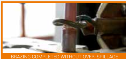
BRAZING COMPLETED WITHOUT OVER-SPILLAGE
